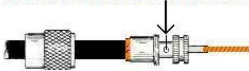
Trim back braided shield wire, but leave about an 1/8 inch. Then continue threading the connector onto the coax until the remaining shield is just inside the connector. Then STOP!
