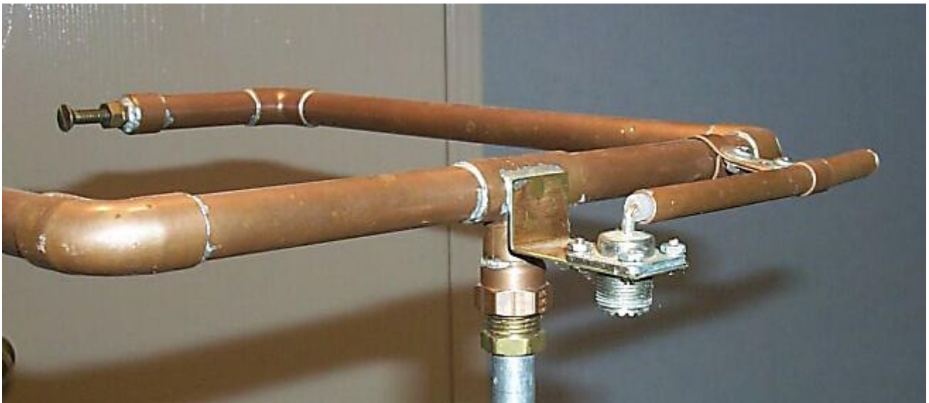
Gamma Match Closeup
