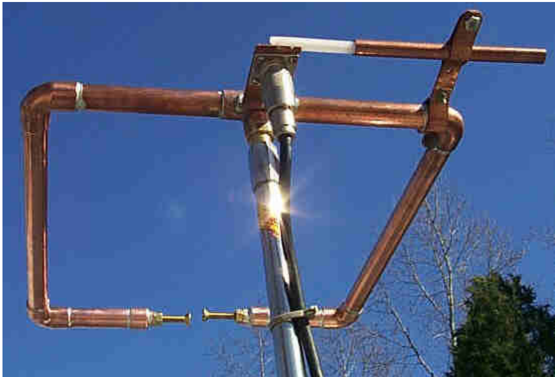
Gamma Match Closeup
