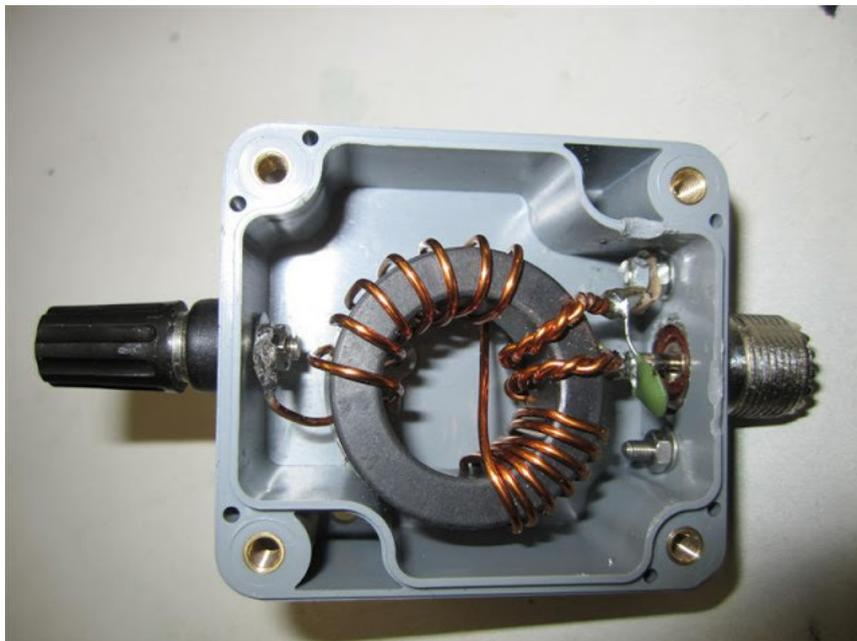
**Transformer made by Tony PA3GWO on a smaller FT140-43 toroid for max. 100 Watt pep**
