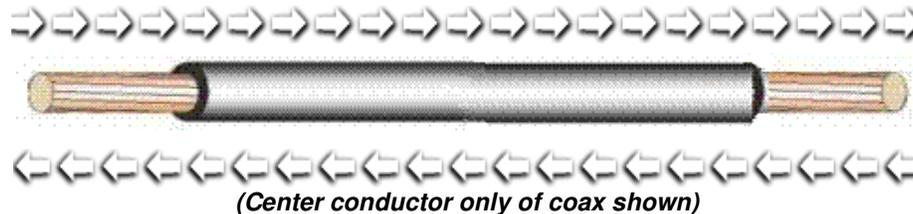
**Rf moves both ways in center conductor of coax!**
