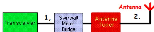
1. above is coax 1 between radio and swr meter
